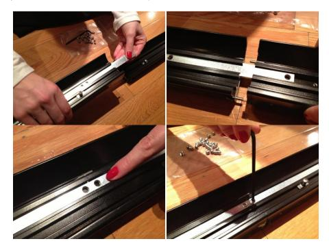
**Install L-brackets.** Align the corner L-brackets into their mating slots in the other frame member, two per corner, and slide them together making a nice tight corner.
