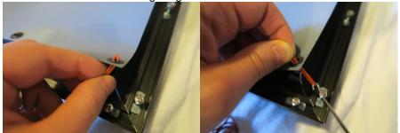
3. Hold top end you poked through, hook with bottom end with tool and loop over post.
