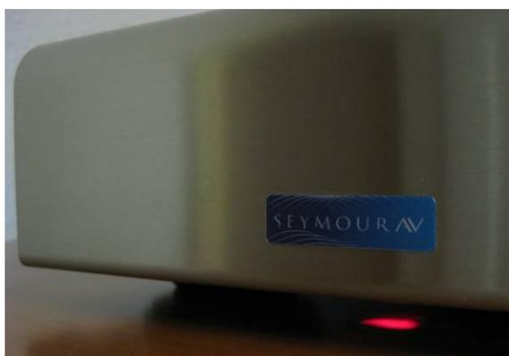
The indicator is an ultra-high brightness red LED that fires indirectly from inside the case, preserving the styling of the amp. The red light is easily visible with a reflective or light colored surface under the amplifiers. Dark non-reflective surfaces, or situations where the front of the amp is hanging off the shelf may not give the LED anything to bounce off of.
