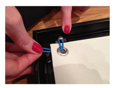
Repeat this process around the screen. You can install the o-rings in any order or pattern you want. The constant tension will actively center the screen and correct for any misalignments. We've installed the screw posts to a tolerance of +/- 0.25", which is fine for the self-centering nature of the o-rings. If you want to adjust the location of any screw post, it's easily done with a Philips driver. Simply loosen, slide in the track where you want it and tighten.
