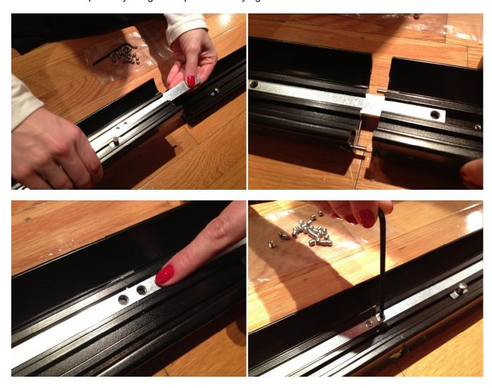
**Install L-brackets**. For the top, bottom and one side frame piece, align the L-brackets into their mating slots in the other frame member, and slide them together making a nice tight corner. It's easiest to save the other side piece for last. Don't tighten screws yet.
