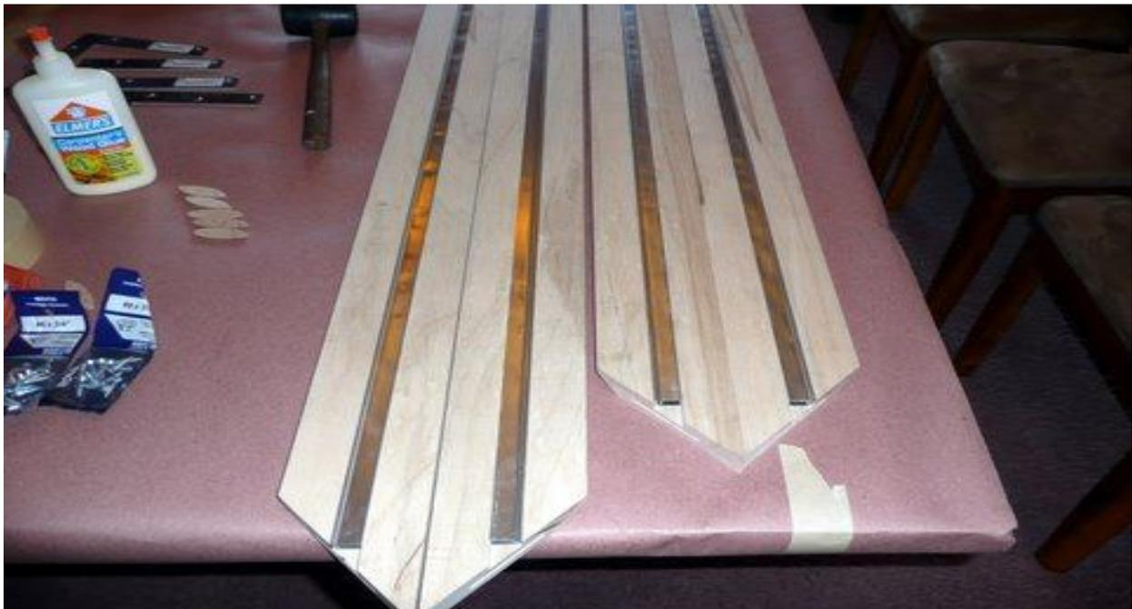
Next, tape over the metal tracks and trim the tape to the width of the rails with a razor knife, then flip the boards over so the viewing side is facing up.
