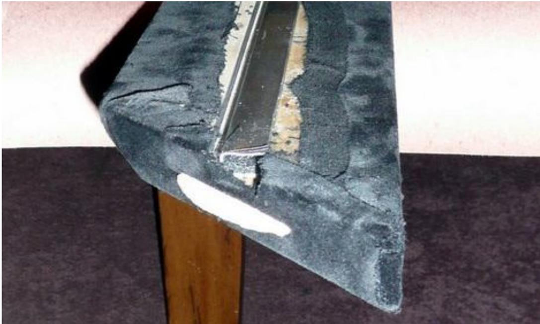
Carefully spray adhesive and tack down the end excess to the back. If you biscuit jointed the edges, carefully slice open the slot and insert the biscuit. You won't need to glue the biscuit in as the velvet will hold it in place nicely. Repeat this process with the other 3 frame sections.
